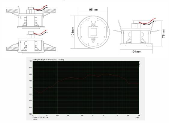
**Features:**Small caliber indoor ceiling speaker, using 3 inch full frequency high-quality speaker unit, high-grade and beautiful appearance, movable clip design, easy to install.
