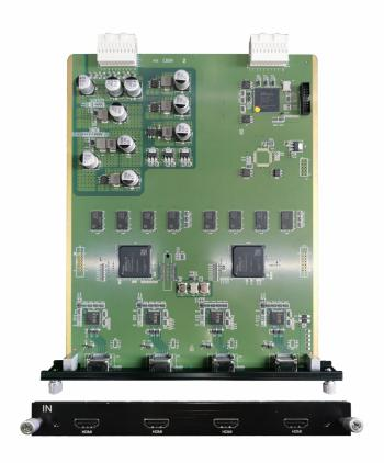
**Description:**The 4-channel HDMI input card is a HD image input board card of LED image processor, which can support 4 channels of HDMI digital signal inputs. It also supports HDCP and EDID functions, and the maximum resolution of 1920\*1080P.
