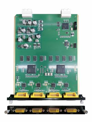
**Description:**The 4-channel DVI output card is a HD image output card of LED image processor, which supports 4 channels of DVI HD digital signal outputs, and also supports EDID function.
