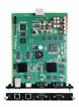
**Description:**The hardware echo output card and control card supports visual recognition of the input signals. And the current display state of the system can be checked on the monitor, which has smooth and clear preview and echo interface, and image echo refresh speed of greater than 30Hz. It also supports dual control card hot backup.
