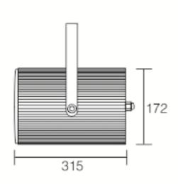
\* Build in straight horn, aluminum alloy structure, anti-rust and anti-corrosion, it can adjust angle arbitrarily and choose multi-power. Suitable for station such as railway station, bus station, etc.
