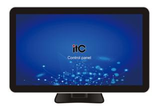
**Description:**TS-9121 is one 21.5 inch desktop capacitance touch panel, match with programmable central controller, HD resolution 1920x1080P, elegant appearance, support wired connection, particularly applicable to anti-leaks place, capacitance touch mode, the front panel of toughened glass is explosion-proof waterproof splash, support programming pictures, graphics, tests, 2D/3D buttons and so on more humanized interface, support picture in picture display.
