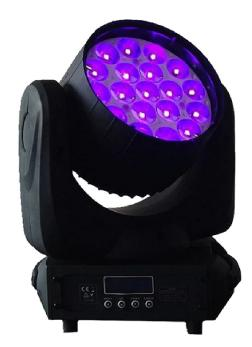
Feature: \* Dimming: 0-100% linear adjustment. \* Color mixing: RGBW stepless color mixing. \* Strobe: 1-25 times/sec (conventional strobe, thunder strobe, random strobe, suddenly dark gradually brighter strobe, suddenly bright gradually darker strobe). \* Scan range: X-axis 540 degrees, with self-recovery closed-loop system; Y-axis 270 degrees, with self-recovery closed-loop system. \* Scanning fine-tuning: X/Y axis 16BIT scanning subdivision for accurate positioning.
