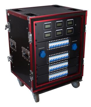
**Feature:** \* Adopt a 225A main switch and a high breaking air switch with double protection of overload and short circuit. \* 3-phase independent voltage, current and monitoring; 3-phase A.B.C indicators. \* Three output modes: 40A bakelite plug, 16A waterproof plug, 19-pin plug. \* Dimension: International standard 14U.
