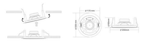
**Description:**High quality ceiling speaker, plastic basin frame, spring pressing system, convenient installation. It is suitable for hotels, hotels, clubs and so on.
