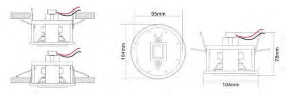
Description: Small caliber indoor ceiling speaker, using 3 inch full frequency high-quality speaker unit, high-grade and beautiful appearance, movable clip design, easy to install.
