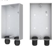
Box Dimension (L×W×D):123×72×32mm Wall Opening Size(LxWxD):126x75x31 mm
